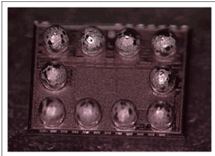
Figure 2. A 12-bump chip-scale package, 3 × 4 bumps, with 2 bump locations not populated.
