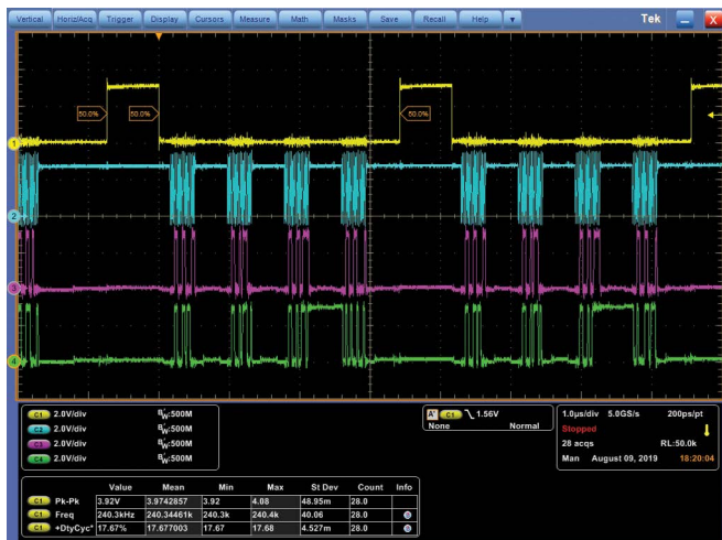
Figure 13. Scope capture of AD7606B BUSY, SCLK, and data on DOUTA and DOUTB.
