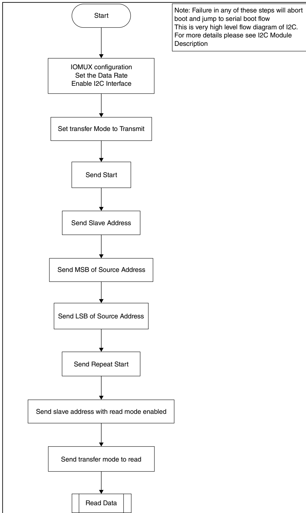
Figure 7-22. I2C Boot Flow Diagram
